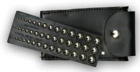
Chrome alloy steel balls, plus/minus .0001" diameter, .000.025" sphericity.
