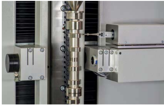
Tactile measuring unit with y-measuring axis 60 mm
