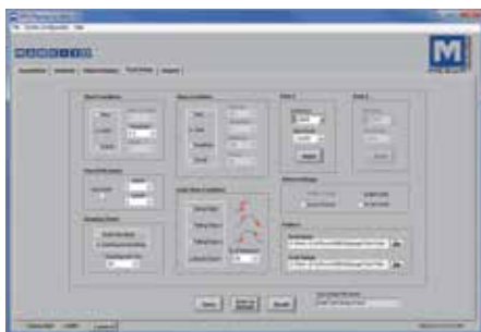
▲ Configure start and stop conditions, such as load, break, time, or distance. Select either discrete data point collection or continuous data collection at up to 50 Hz.
