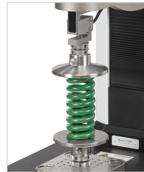
Compression spring testing
