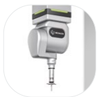
Digital touch trigger probe DTT
